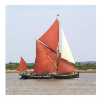
Built in 1922 by London & Rochester Trading Co., Pudge is a Thames sailing barge with a hull constructed of pitch pine on oak with a flush deck, with the steering wheel on a 'short spindle' without the usual raised cabin top. Originally spritsail rigged with a bowsprit she had an auxiliary oil engine made by The Bergius Co. Ltd of Glasgow and was installed in 1932. Pudge is one of the last wooden barges to be built,
